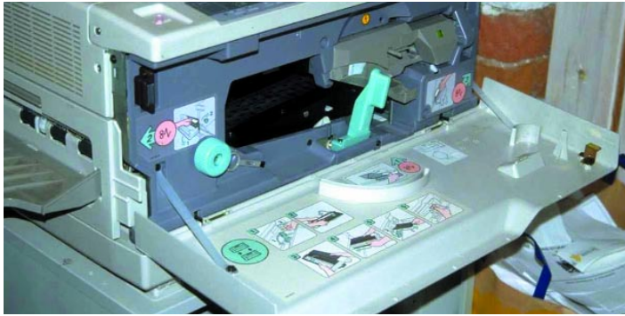
This Xerox mashine at my work had controls and levers that were designed so that you immediately understood which way to turn them.
